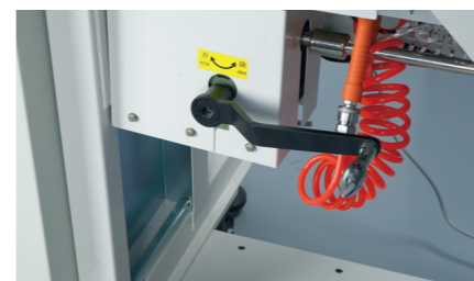
标配可升降调节机架 Standard configuration can be raised and lowered to adjust the rack
